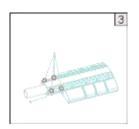
3. Mount the luminaire onto a pole. Tighten up the screws to fixate it.
